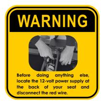
**NOTE**: If you forgot to disconnect the 12-volt power supply, you will need to replace the fuse in the power adapter with a new one provided in the tool case. To do this, unscrew the end of the power adapter, remove the old fuse, and insert the new one.
