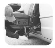
There are four (2) holes under the trim on the front of the unit. The two outer holes move the TRAVEL motor and the two inner holes move the TILT motor. The third motor is the PIVOT and it can be found at the back of the LINK. (Shown far right: The backup tool has been designed to curve for the pivot motor, in case your vehicle is equipped with a center console.)
